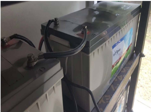
Figure 7.3 Swollen inverters batteries caused by exposure to high temperatures
